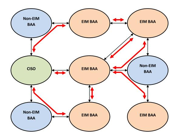
EIM BAAs may be interconnected with the CISO directly, through another EIM BAA, through a Non-EIM BAA, or a combination thereof. The EIM Entity for an EIM BAA may have made available transmission rights on a direct interconnection with the CISO, on a direct interconnection with another EIM BAA, or on an indirect interconnection with the CISO or another EIM BAA through one or more non-EIM BAAs.
